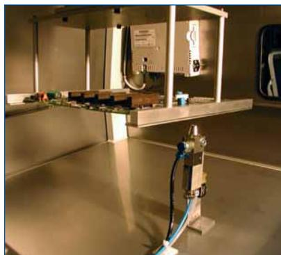
*Fig 3: Example of a Spray Fluxer Head*
