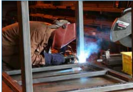
*Fig 8: All-welded construction*
