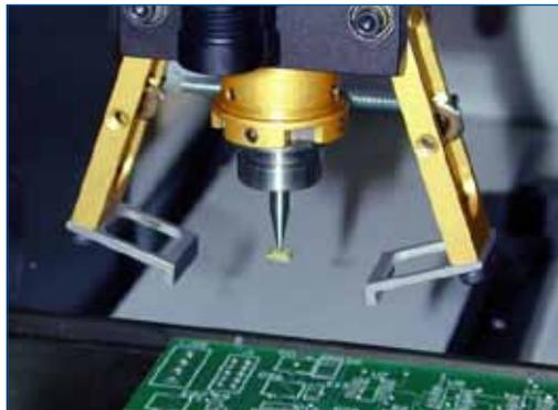
*Fig 4: Mechanical Centering*
