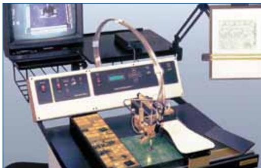
*Fig 3: A vision-assisted manual machine*
