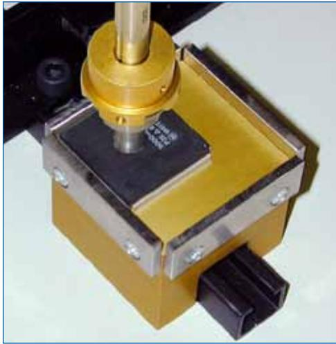
**3. Method 3: Laser centering** In this method, the component is picked up inline with a laser beam which detects the component's center position on the tool head and recalculates the zero point of the part according to its position in the X, Y axes and rotational position relative to the head for an accurate placement on the board.
