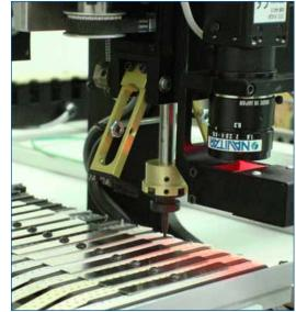
Fig 9: Work deck with component feeders
