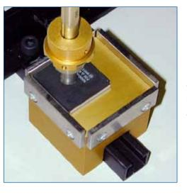
**3. Method 3: Laser centering** In this method, the component is picked up inline with a laser beam which detects the component's center position on the tool head and recalculates the zero point of the part according to its position in the X, Y axes and rotational position relative to the head for an accurate placement on the board.
