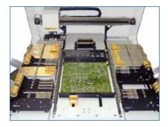
**Method 1: No positioning feedback loop** In this system, the motor drives the part to a location on the board defined in the program by the number of steps in each X-Y axis, but there's no way to tell if it actually ends up in the right place. These systems use stepper motors for positioning.
