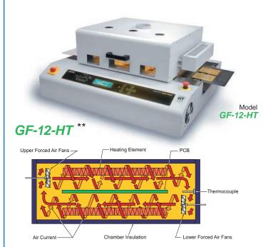
Our patented Horizontal Convection<sup>TM</sup> technology\*\* circulates heated air in each chamber around the board front to back which increases the thermal efficiency and uniformity within each zone. This exposes the circuit board to a uniform temperature profile along the entire assembly. Cyclonic generator speed is independently set in each zone.
