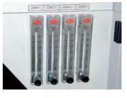
All GF ovens have a nitrogen gas inerting option. With the isolated chamber design (recirculation of atmosphere within reflow zone) low oxygen levels are maintained while conserving nitrogen consumption.
