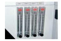
Novastar's isolated chamber design (recirculation of atmosphere within each chamber) maintains low oxygen levels while conserving nitrogen.
