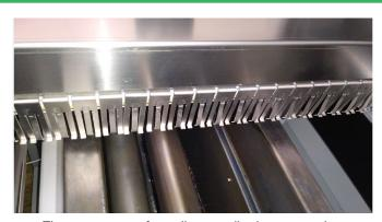
Finger conveyor for pallet or pallet-less operation.
