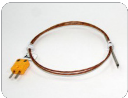
A-0234-15 Thermocouple, K Type Thermocouple With Extended Tip - Models 1800,2000, GF-120, GF-12, GF-B
